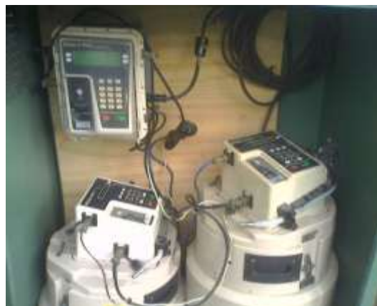
Figure 6. An example of the autosamplers used for wet weather water quality sampling. Two samplers were required for the samples analysed.
